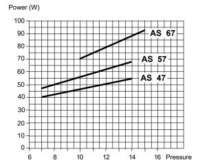
Viscosity = 5 cSt - Rated speed = 2850 rpm (bars)
